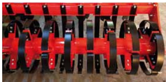
Spring roller Ø540mm DiscoMax, Dracon
