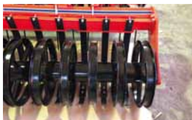
U-roller Ø540mm DiscoPlus, DiscoMax, Dracon
