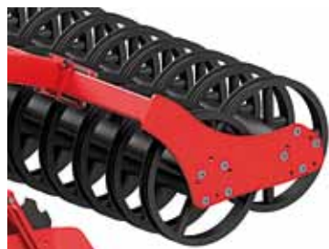
Double U-roller 2 x Ø540mm DiscoPlus TR, DiscoMax RT, Dracon RT
